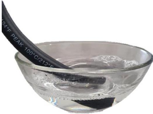
For even easier assembly, use soapy water as lubricant. Simply dip the end of the hose in the soapy water beforehand, and dry off the outer surface of the hose before assembly
